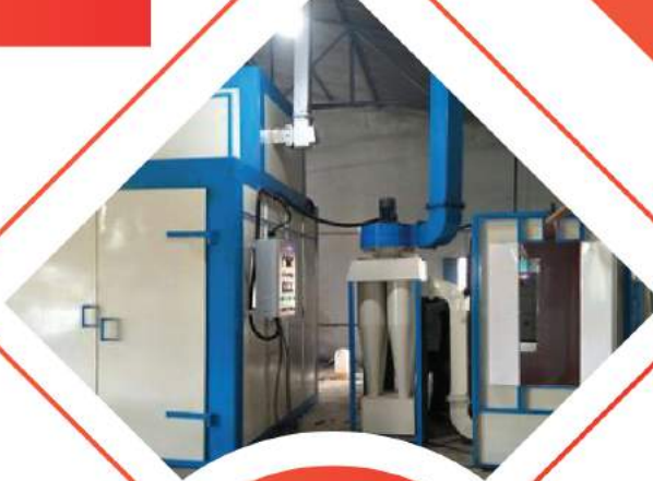
Powder & Paint Coating Curing Oven
